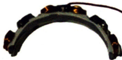
Figure 7: Alternator stator of the 5 hP gas engine (Removed)
