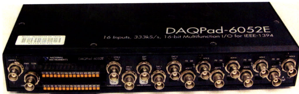
Figure 24. Photograph of the National Instruments Data Acquisition Unit, the DAQPad 6052e. This device contains digital I/O lines and analog input and output ports.
