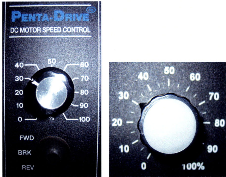
Figure 3-2 Control panel to adjust feed rate (left) and vibratory feeder frequency (right)
