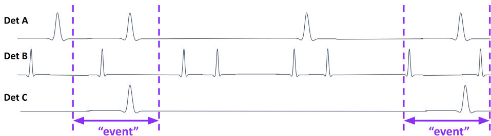
Figure 3. Traditional triggered systems record regions of time surrounding a possible interesting physics interaction as an “event”. This sketch illustrates this. For streaming mode, the concept of an “event” transitions into a time frame. See text for details.
