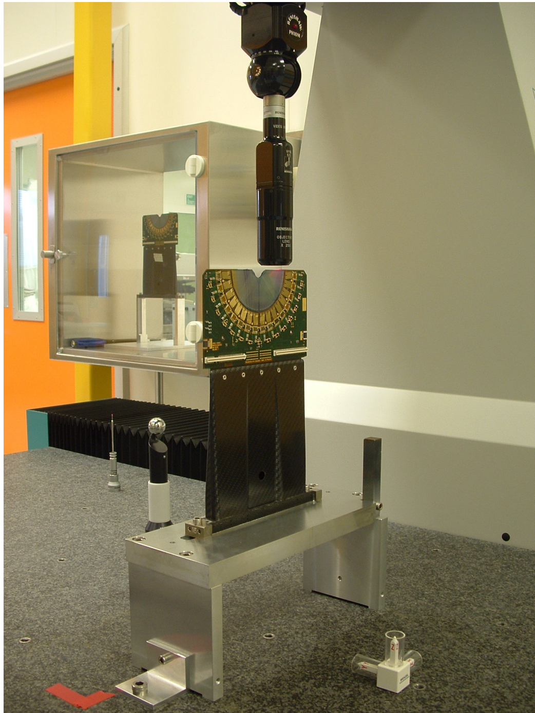
Figure 1: View of Module and Pedestal on Jig Base with Optical Probe
