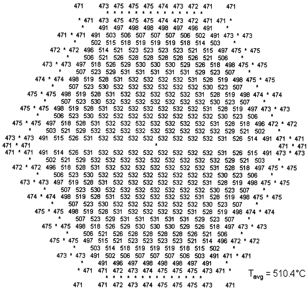
Figure 3.20: Core outlet temperatures for subchannel analysis using SUPERENERGY II at the heated length outlet
