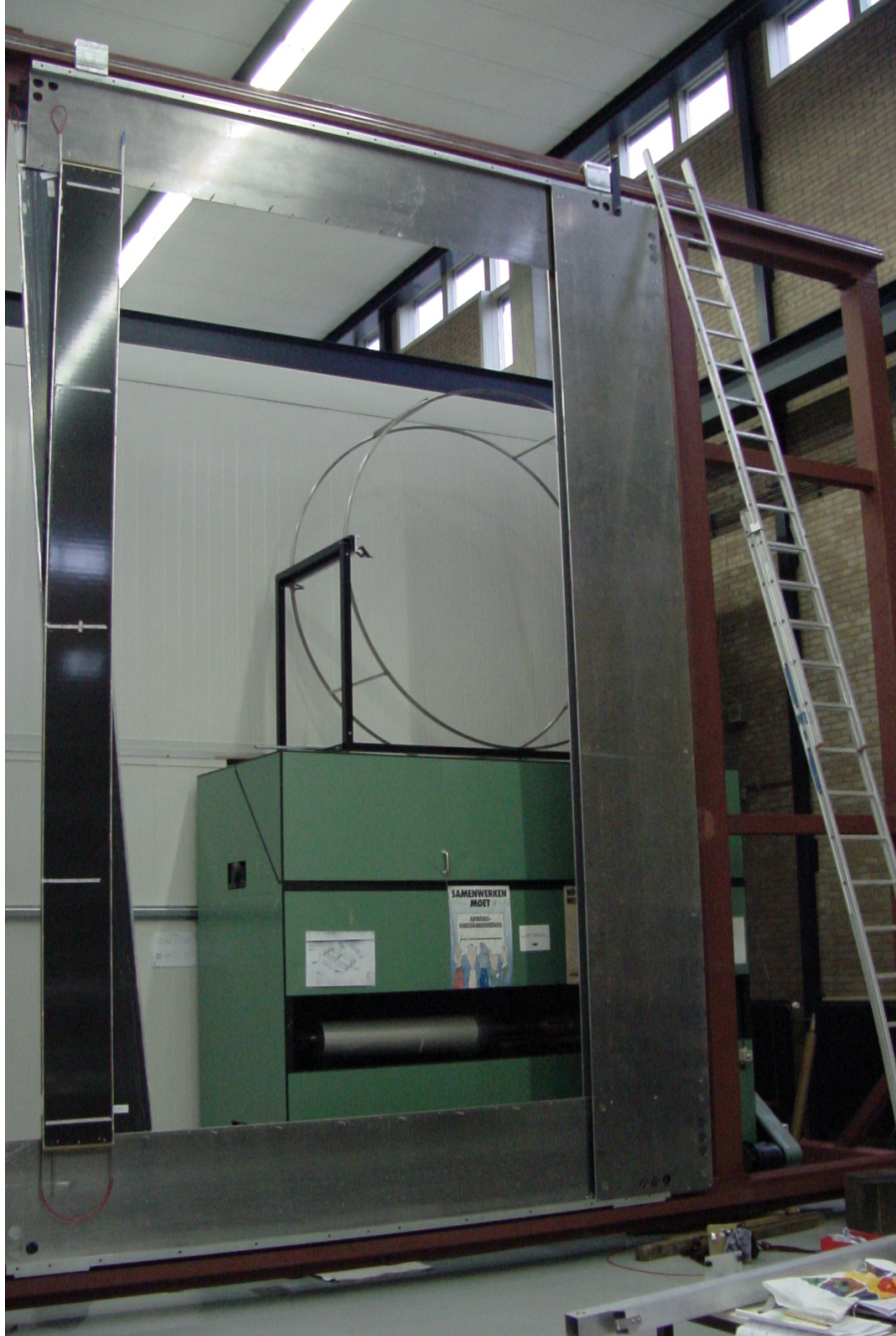
Figure 1.2: Two LHCb Outer Tracker modules in two different layers in a C-Frame. In the actual LHCb setup, the Outer Tracker will consist of 12 C-frames, six on either side of the beampipe
