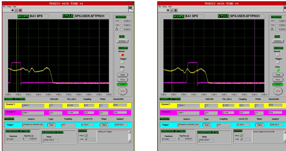
Figure 13: Snapshot of the LabView scope startMopos: in yellow (white in b/w) the sum BPM signal showing the 10.5 \mu s long batch, in magenta (gray in b/w) the BPM gate moving from the fourth slice (left) to the fifth slice (right). Note that the timebase is here set to 1 \mu s per division and the Trig. Pos is set to 9 \times 10^6 .
