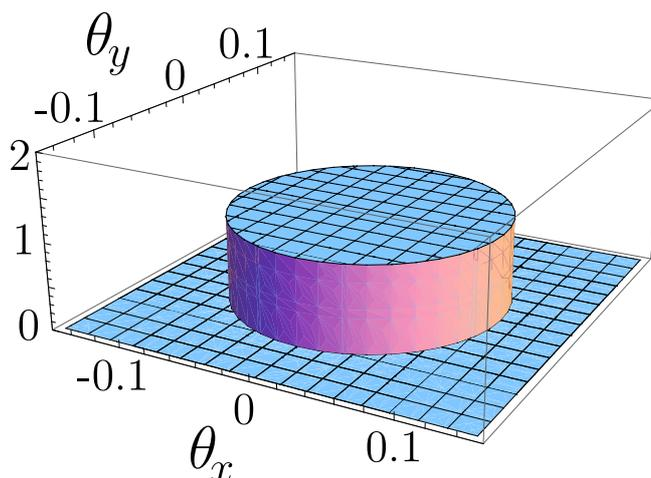
**Figure 13:** The angular ordering approximation. The function  $g$  defined in eq. (4.15) and plotted in figure 11 is replaced by the function  $g_{\text{a.o.}}$ , eq. (7.11), plotted here. The plot coordinates and value of  $\theta_{lk}$  are as in figure 11.
