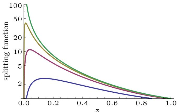
**Figure 3:** The spin averaged splitting function  $F$  defined in eq. (2.23) for a final state  $q \rightarrow q + g$  splitting, plotted versus the momentum fraction  $z$  of the gluon, as defined in eq. (2.20). The quark is taken to be massless and we set  $a_l = 4$ . The four curves are for, from bottom to top,  $y = 0.03, 0.01, 0.001, 0$ . For  $y = 0$ , the result is the Altarelli-Parisi function,  $[1 + (1 - z)^2]/z$ .
