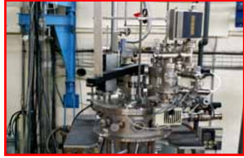
Fig. 3: Photograph of the upper part of the insert ready for cryogenic test.
