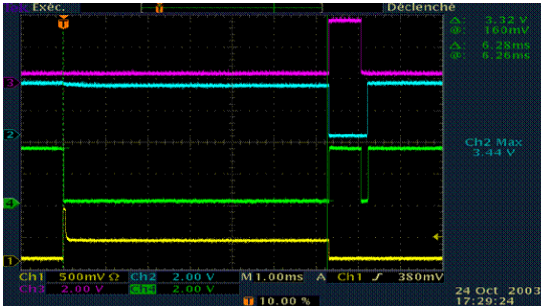
Figure 24: Screen shot of the measurement of the ON, SET and FAULT pins (from top to bottom) and last the command of a load to simulate a SEL.
