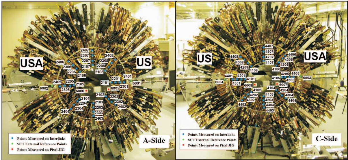
Figure 1: Details of the photogrammetry survey [6]
