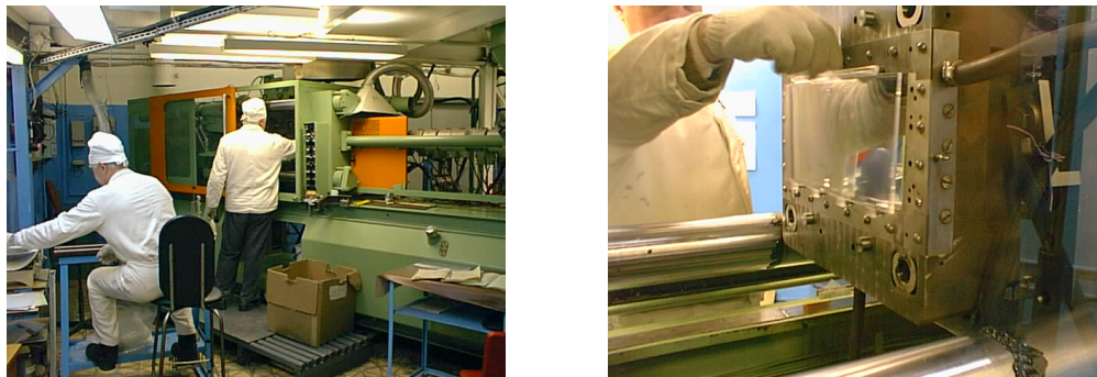
Figure 11: The mold machine (left) and a just molded tile (right).
