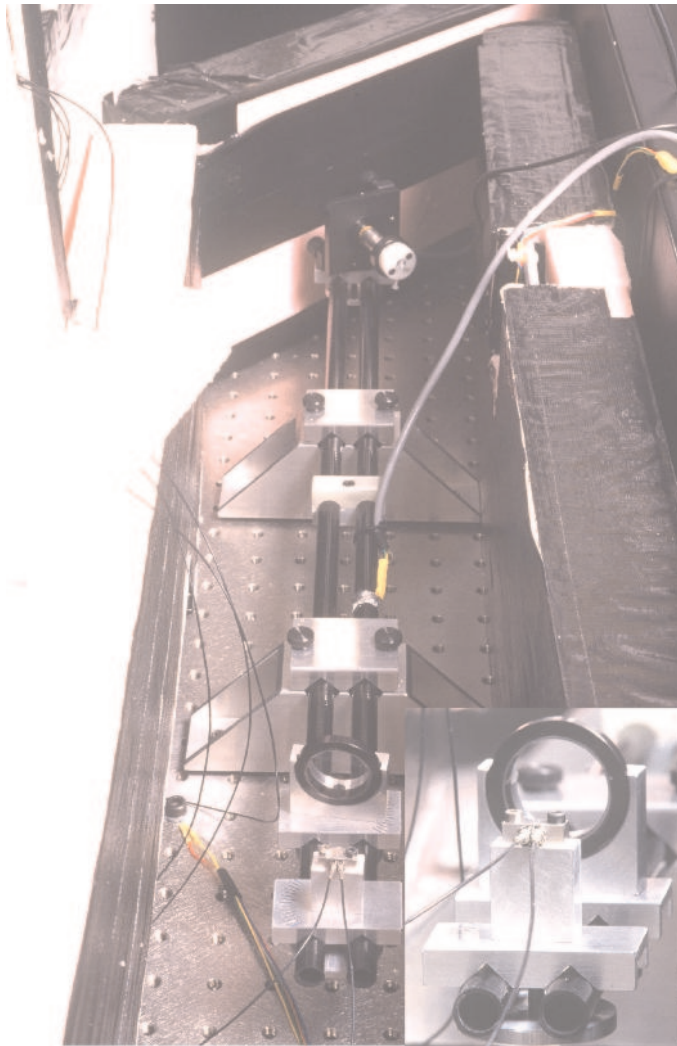
Figure 2.26: A grid line interferometer built on two carbon fibre rods. At the nearest end, the delivery and return fibres point towards the nearby pellicle beam-splitter and the retroreflector, which was mounted on a PZT so that vibrations could be deliberately induced when required. During FSI measurements, the thermal insulation was completed by a polystyrene lid and front wall. INSET: The fibres and pellicle beam-splitter in more detail.
