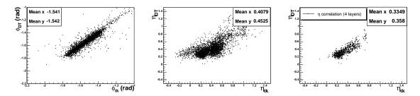
Figure 55: Correlations of directions of tracks, in the absence of magnetic field, reconstructed in the tracker and in the Drift Tubes. The  $\phi$  correlation is shown left. The  $\eta$  correlation for all the tracks (for tracks with hits in 4 layers) is shown in the centre (right).
