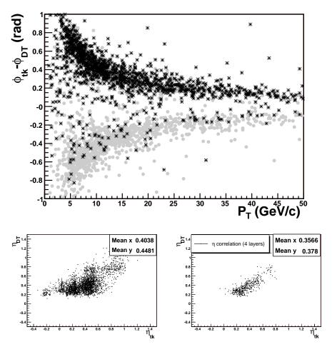
Figure 56: Correlations in the direction of tracks, reconstructed either in the tracker or in the Drift Tubes, at  $B=3.8\,\mathrm{T}$ . The difference  $\phi_{tk}-\phi_{Dt}$  (top) is correlated to the transverse momentum measured by the tracker for positive (black) and negative (gray) muons. The bottom plots show the  $\eta$  correlation for all the tracks (left) and for tracks with hits in four layers (right).
