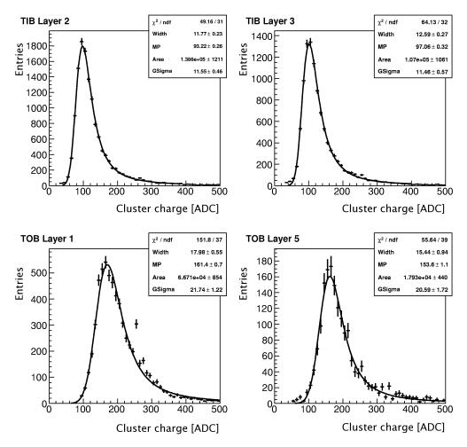
Figure 58: Cluster charge for TIB and TOB modules at B=0 T. The cluster charge is proportional to the detector thickness: nominally 320  $\mu$ m for TIB and 500  $\mu$ m for TOB, though in both cases the active sensor thickness is 20-30  $\mu$ m less.
