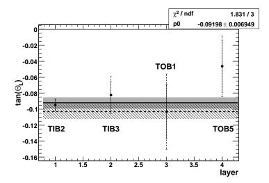
Figure 79: Results of the Lorentz angle measurement in the four different layers using tracks reconstructed by the Road Search algorithm In increasing abscissa value, points correspond to TIB L2 and L3 and TOB L1 and L5. The horizontal line represents the result of the combination of all four layers and the shadow band is the fit uncertainty. The dashed line and the hatched region represent the expected value and his uncertainty, respectively.
