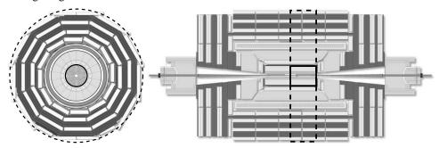
Figure 7: View of the CMS Generator Target region: xy view (left) and yz view (right). Only generated muons that cross the detector in the regions defined by a continous line for the B=0 T and by a dashed line for B=4 T are retained for the subsequent analysis.
