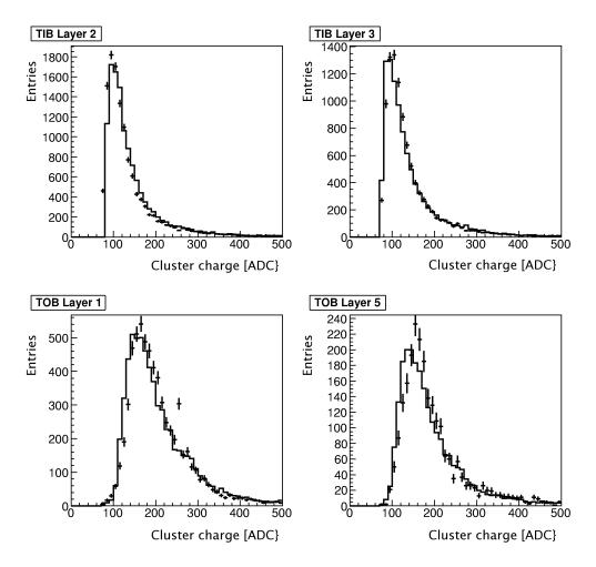
Figure 62: Cluster charge distributions for TIB and TOB at  $B=0\,\mathrm{T}$ . Solid line - MC simulation, points - data.
