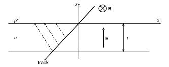
Figure 77: Lorentz drift in the microstrips silicon sensors.
