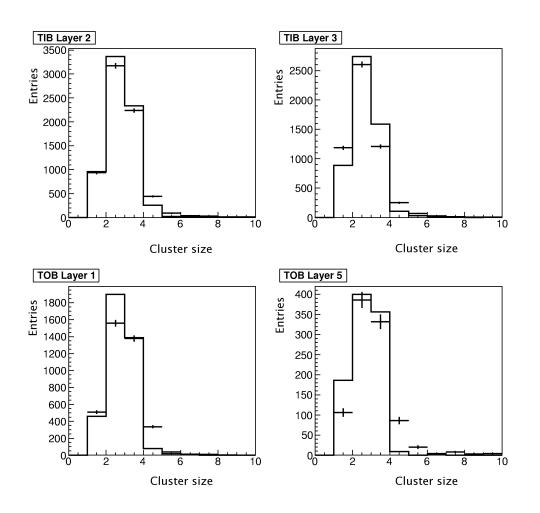
Figure 67: Cluster size distributions for TIB and TOB at  $B=3.8\,\mathrm{T}$ . Solid line - MC simulation, points - data.
