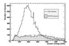
Figure 75: Comparison between CSC and DT trigger (left) or CSC and RPCTB trigger (right), both with a cut on S/N > 10 (B = 3.8 T).
