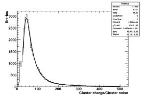
Figure 68: Cluster charge for TEC modules at  $B=3.8\,\mathrm{T}$  (cluster charge < 500). The result of the fit with a Landau function is shown.
