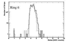
Figure 44: Tick mark height calibrated noise of ring 6 modules for three pedestal runs.
