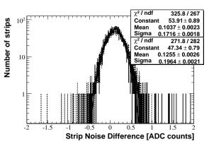
Figure 29: Tick mark height calibrated noise strip difference distribution for layer 1
