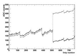
Figure 31: Saturated pedestal module.
