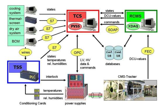
Figure 2: Dataflow in the TCS
