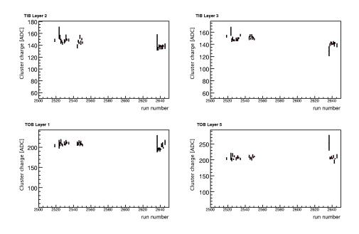
Figure 60: Cluster charge for TIB and TOB vs. run number at  $B=0\,\mathrm{T}$ .
