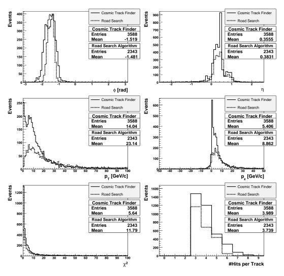
Figure 54: Various track distributions for the Cosmic Track Finder (solid line) and the Road Search algorithm (dashed line) using the  $B=3.8\,\mathrm{T}$  data sample:  $\phi$  and  $\eta$  (top),  $p_T$  and  $p_z$  (middle),  $\chi^2$  and number of hits per track (bottom). The distributions for the Cosmic Track Finder are shown for tracks with hits in at least three layers.
