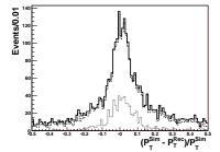
Figure 10: From left to right resolutions of  $\phi$ ,  $\eta$ , and the transverse momentum relative resolution. Resolutions are shown for all the tracks (solid), for tracks with hits at least in three layers (dashed) and for tracks that have hits in four layers (dotted).
