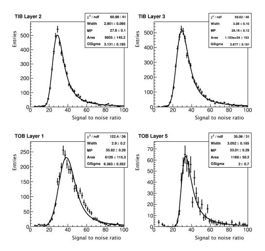
Figure 61: Signal-to-noise ratio distributions of clusters for TIB and TOB at  $B=0\,\mathrm{T}$  corrected for the path length in silicon.
