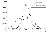
Figure 9:  $P_T$ ,  $\eta$ , and  $\phi$  distribution for cosmic muons in the  $B=4\,\mathrm{T}$  sample, before (plain) and after (dots) the DT trigger selection. All distributions are normalized to unity as relative efficiency of the DT filter for events in the tracker can not be measured on data. The distributions are superimposed to approximately show the change in the distributions when a DT trigger is present.
