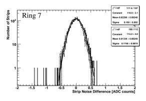
Figure 49: Tick mark height calibrated noise difference of ring 7 modules.
