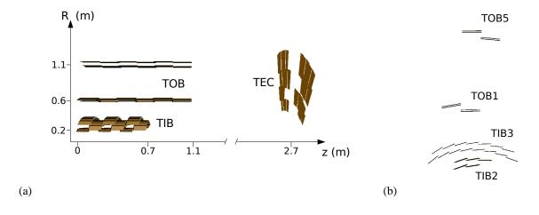
Figure 1: Layout of the Tracker MTCC setup: (a) 3D view (the z axis goes from left to right); (b) xy view of the barrel part. The instrumented parts are a fraction of layer 2 and layer 3 of TIB, two rods in layer 1 and in layer 5 of TOB, two petals in disk 9 of TEC.
