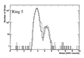
Figure 43: Tick mark height calibrated noise of ring 5 modules for three pedestal runs.
