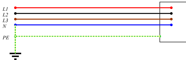
Figure 3: TN-S distribution scheme for the back-end system.
