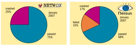
Results of vulnerability tests performed by CERN on PLCs using standard penetration tools.
