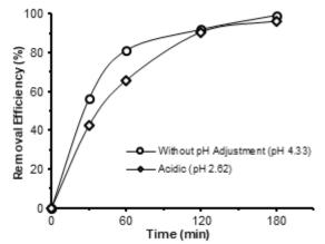
**Fig 1.** Removal efficiency of copper ions by CSAC electrode at acidic condition (pH 2.62) and without pH adjustment (pH 4.33)
