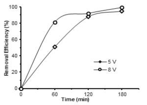
**Fig 2.** Removal efficiency of copper ions by CSAC electrode at applied voltage of 5 and 8 V
