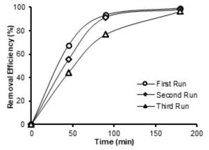
Fig 4. Successive copper ion removal efficiency of CSAC
