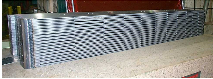
Figure 16: A finished standard submodule.
