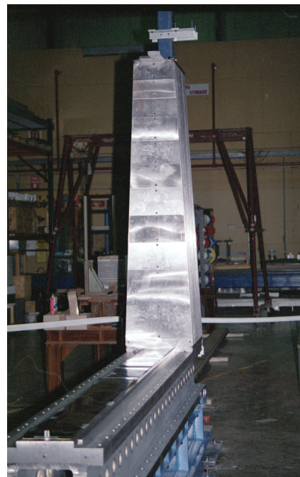
Figure 18: The assembly base used for extended barrel module construction (left). The module alignment system, used at one of the extended barrel module assembly sites. It couples the alignment of the girder via survey pins to the plate inserted at the inner radius of the module and a survey mark and plumb-line on a fixed support placed behind the module (right).
