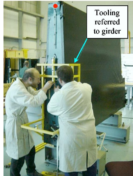
Figure 21: Mounting fiducial marks on the endplates of completed modules for use in surveying module positions during final assembly
