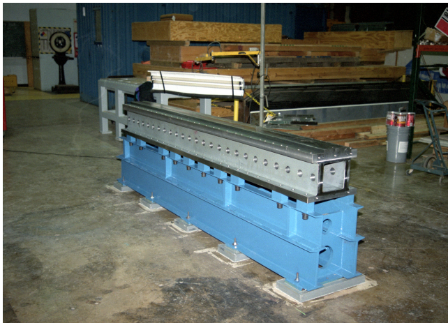
Figure 18: The assembly base used for extended barrel module construction (left). The module alignment system, used at one of the extended barrel module assembly sites. It couples the alignment of the girder via survey pins to the plate inserted at the inner radius of the module and a survey mark and plumb-line on a fixed support placed behind the module (right).
