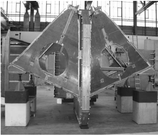
Fig. 7. Sub-assembly of lower coil with two keystone boxes.
