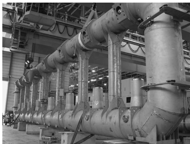
Fig. 1. The individual Barrel Toroid coil has passed the on-surface test in the ATLAS Magnet Test facility and is being prepared for the transport to the underground area of the ATLAS experiment.
