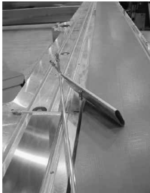
Fig. 3. View of a bladder on top of a double pancake inserted in the coil casing. The cut bladder has been inflated and is already 3 times thicker than before inflation. One bladder is already inserted in the gap between the coil casing and the double pancake winding.
