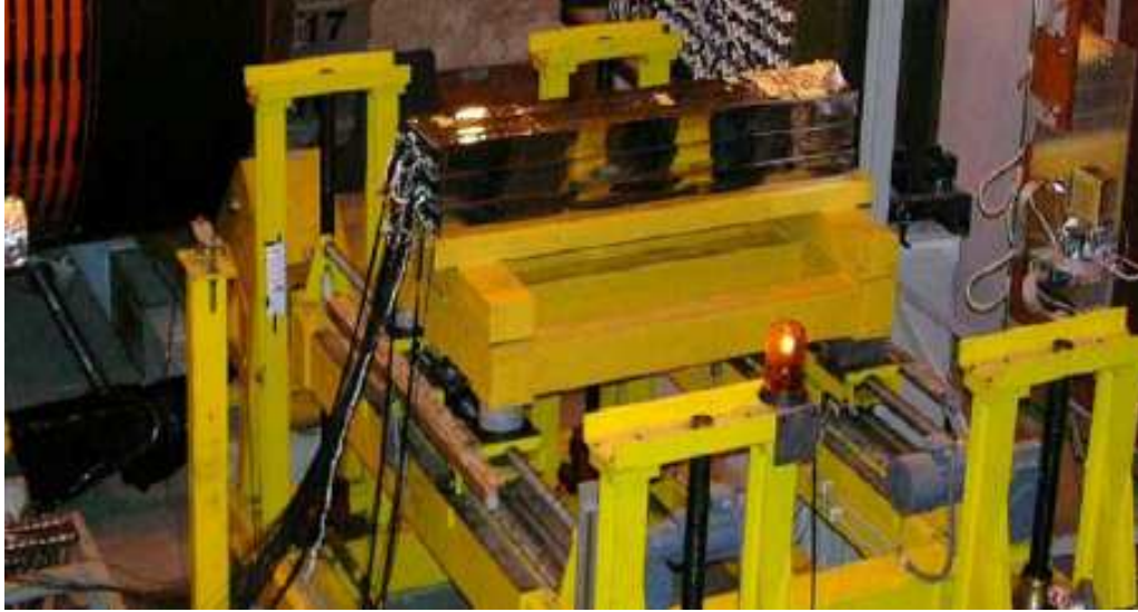
Figure 4: The PSD super-module positioned in the NA61 experiment downstream of the MTPC hut.
