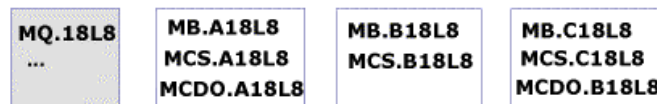
Figure 7: Naming Convention for Magnets in a Standard Half-cell with 1 LBB assembly and 2 LBA assemblies
