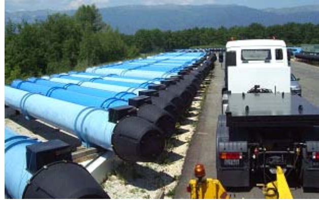
Figure 2: Part of one of the cryo-dipoles storage area – the picture shows approximately the number of cryo-dipoles installed during one week.
