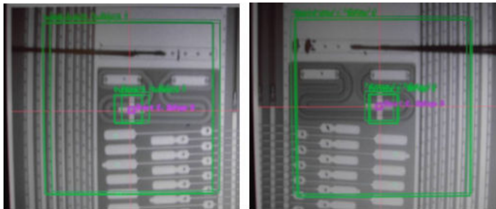
Figure 8: Fiducial marks for the sensors used to define the references 5 to 8. These are in identical positions for both the r and phi sensors.
