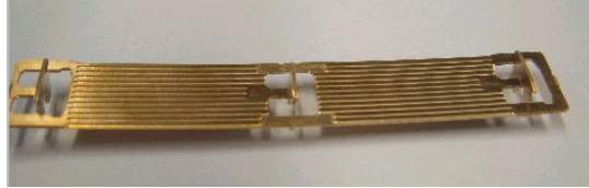
Figure 2: Clamp seat with ears bent to shape and lugs protruding below. The engagement side is uppermost
