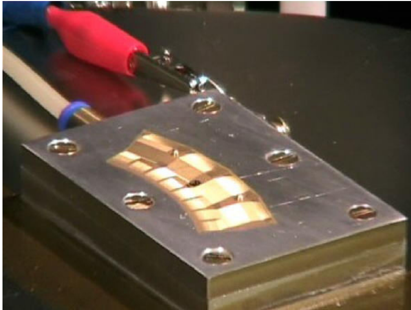
Figure 4: Photograph of pitch adaptor on its testing jig.
