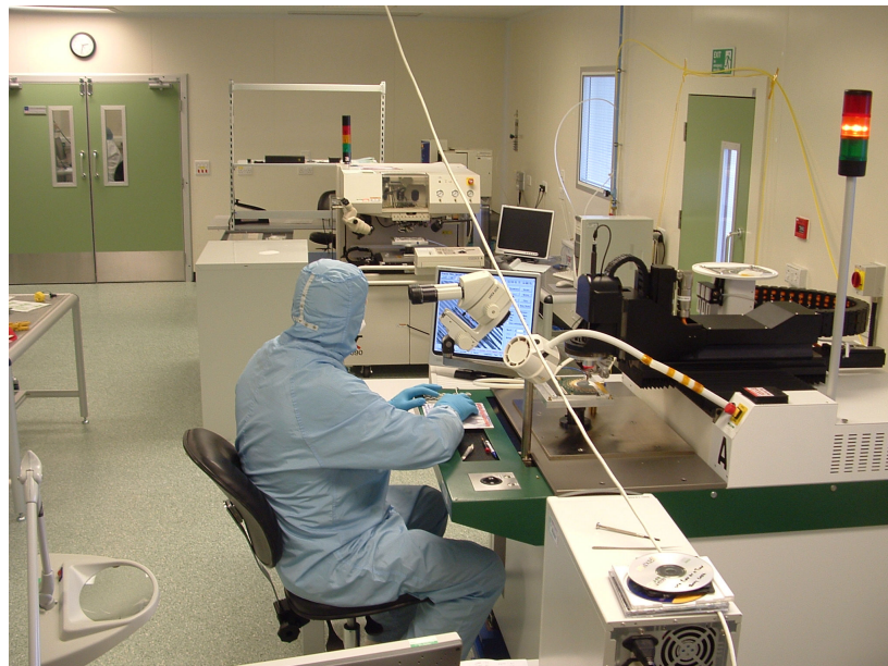
Figure 5: View of bonding zone showing H&K. The K&S 8090 can be seen in the background.
