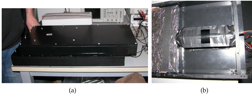
Figure 4.3: (a) Photo of two 1 \times 20 \times 30 \text{ cm}^3 scintillators; (b) detail of the photomultiplier coupled to the scintillator.
