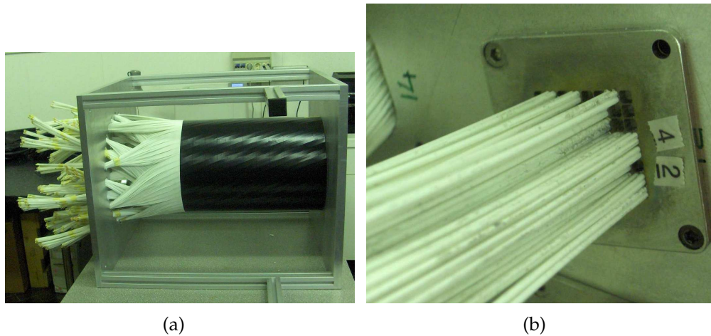
Figure 3.2: FAST tracker assembly: (a) all scintillating fibers have been placed on the supports and grouped to match the 42 PMTs; (b) detail of the iron mask to couple the fibers to the 64 PMT anodes.
