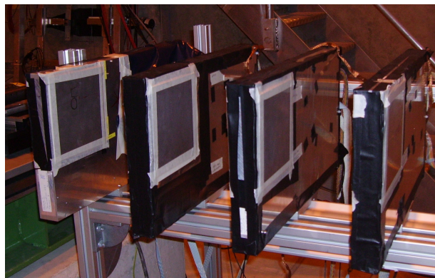
Figure 3.5: The 4 x-y silicon chambers in the downstream region.
