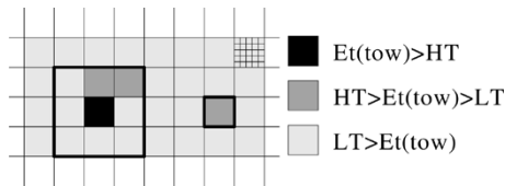
Fig. 1. Selective readout algorithm. See the text for the description of the algorithm. The figure illustrates the case of one trigger tower with a high transverse energy deposit (above the higher threshold HT, in black): the crystals of 3 \times 3 trigger tower matrix around this trigger tower are read with a minimal zero suppression threshold. The crystals of the trigger tower with a medium transverse energy deposit (between the higher and lower thresholds, HT and LT, in dark gray) are also read with a minimal zero suppression threshold.
