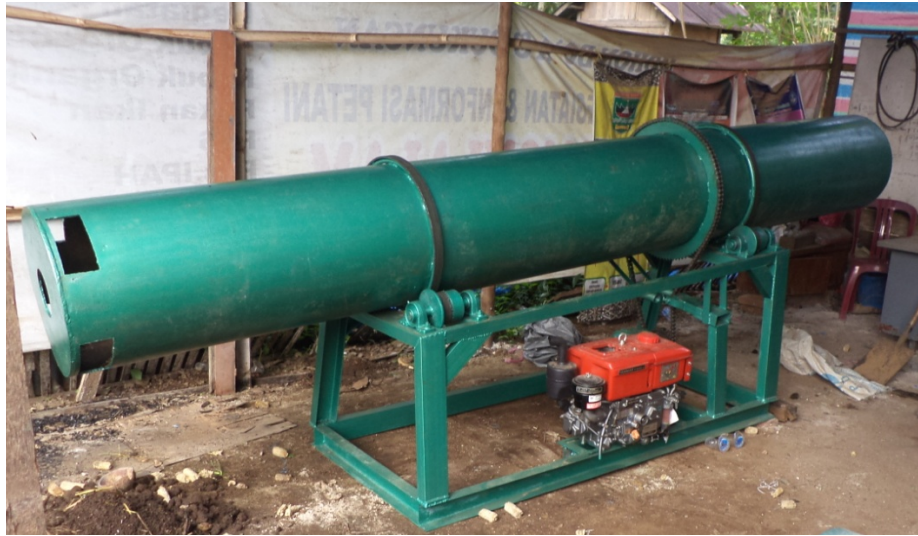
Figure 2. Cylinder drying unit
