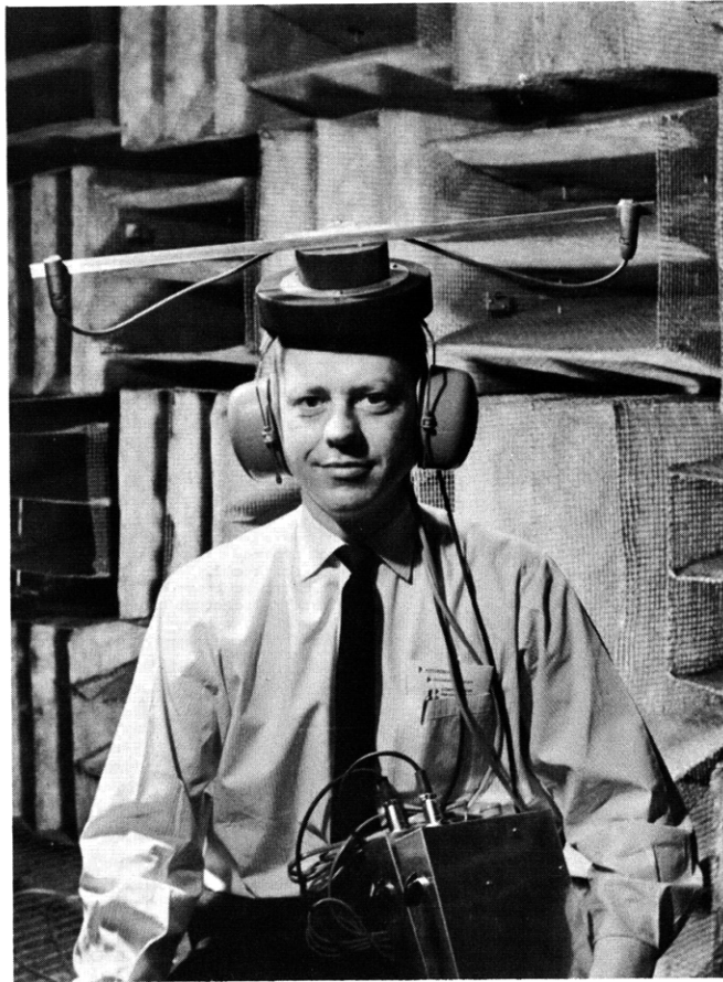
Fig. XIX-17. Apparatus used for "head-stretching" experiment. Signals are picked up by microphones at end of the horizontal bar, amplified by circuitry in boxes, and presented to subject through earphones (unseen) contained in acoustical ear muffs.
