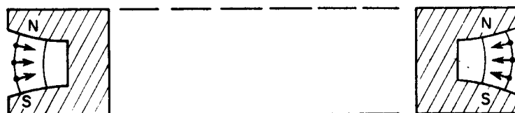
Fig. 4. Cross section of a constant gradient synchrotron ring illustrating focusing
