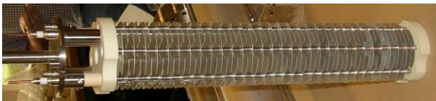
Figure 1: Photograph of the inside of an ionisation chamber. The stack of aluminum electrodes with the insulator ceramics at both ends can be seen.
