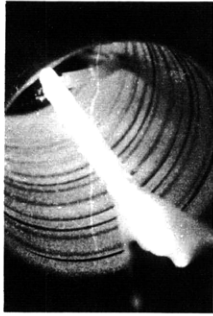
Fig. VIII-9. Spiral instability brought to rest by gas flow in an argon plasma column.
