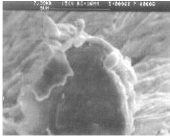
FIGURE 14 Trace of molten crater on a processed surface.
