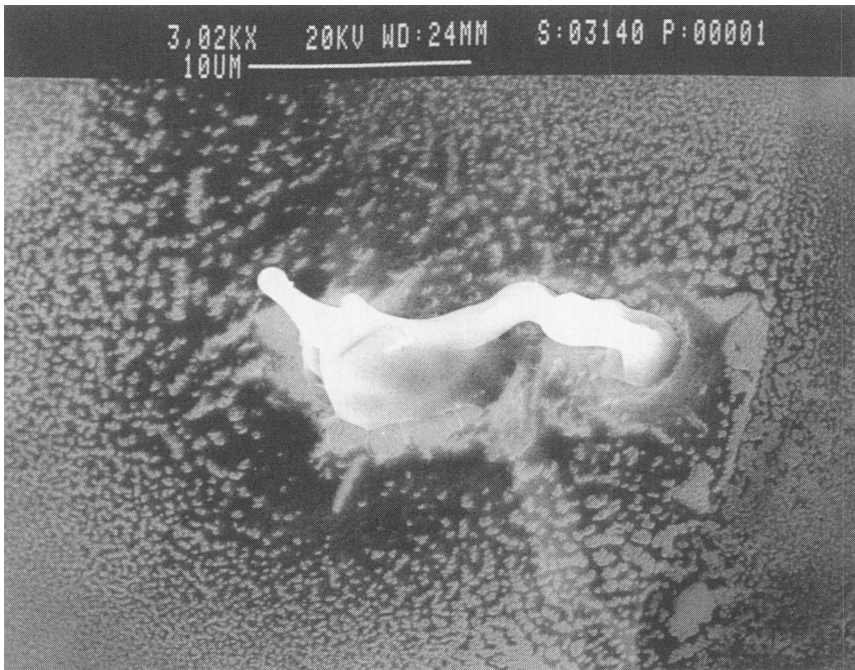
FIGURE 24: SEM micrograph of a dimple tested in the mushroom cavity showing a teflon particle. Note the melted ends. The peak surface electric field at this particle was \sim 40 MV/m.
