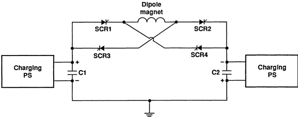
FIGURE 2 Self-Commutating Bipolar Capacitor Bank and Silicon Controlled Rectifier System.
