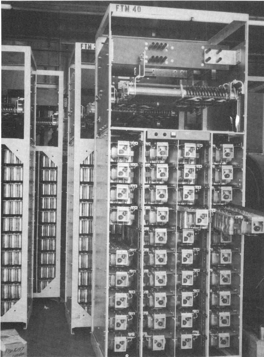
FIGURE 5 Six-MJ Electrolytic Capacitor Bank for Magnetic Fusion.
