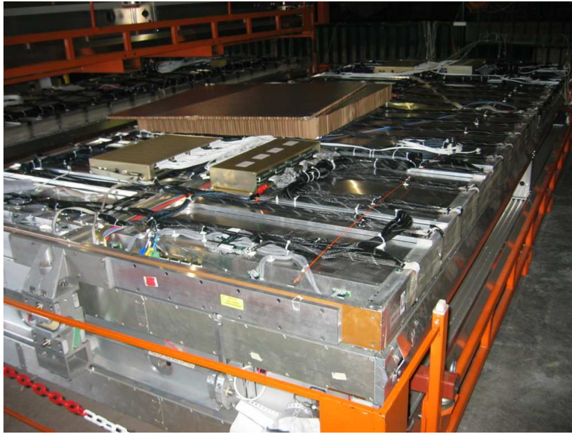
Figure 6.5: Photo of a barrel middle muon station: two RPC are assembled with a MDT, the drift tubes are visible between the RPCs. The boxes mounted on the RPC contain the LVL-1 trigger electronics.
