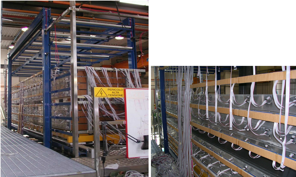
Figure 3.1: Photo of the cosmic test stand at the INFN Roma Tor Vergata Laboratory . Two blocks of four superimposed biggest RPC units can be hosted. Up to 3854 channels are read out.
