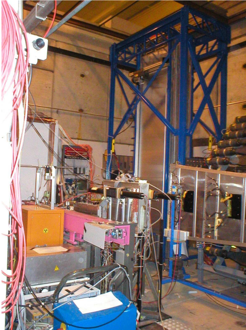
Figure 4.7: Experimental setup at X5/GIF. The chambers under test are visible in the background, in their blue support structure. The orange box in the foreground contains the source, while the pink structure supports the lead filters.
