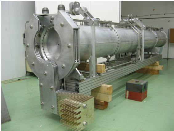
Figure 3: The CNGS horn, before installation in the target cavern.
