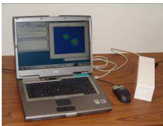
Figure 2. Picture of the mini Gamma Camera prototype with its associated computer.
