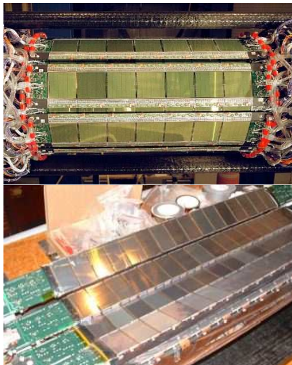
Fig. 3.1: The fully assembled SVT detector (above). One can see the arrangement of the wafers in a ladder. The bottom part of the figure shows one (out of four total) SSD sector. The double-sided strip detectors are also arranged in ladders.
