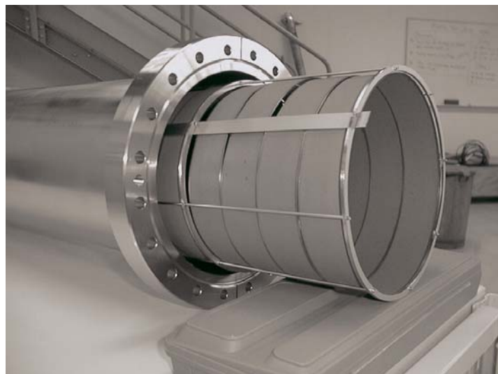
Fig. 4: Schematic view of the St 707 'total' NEG pump
