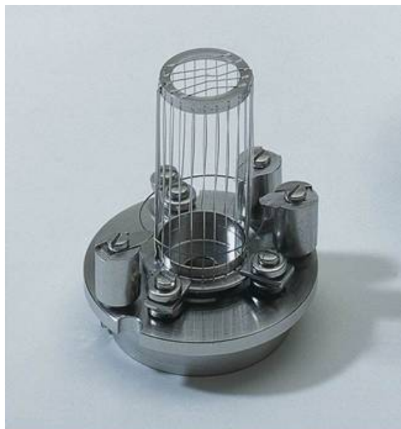
Fig. 15: Grid ion source. The surface of this ion source is minimized by the grid design of the formation chamber.
