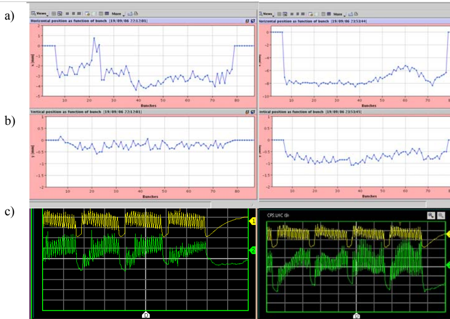
Figure 9. Instability observed in the PS for the nominal LHC beam: a) horizontal and b) vertical bunch position vs. bunch number at the first turn in the SPS. c) Sum (yellow) and horizontal delta signal from a wide-band transverse pick-up in the PS over the last four turns before extraction. In the cycle shown in the left column only a few bunches are affected while in that represented in right column several bunches are affected. Courtesy of R. Steerenberg.
