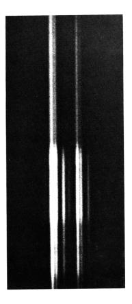
Fig. V-1. The 5350 A line of thallium. The components from left to right belong to isotopes 205, 203, 199, 200, 205, 203, and 199, respectively. The upper part of the picture is the Tl<sup>203</sup> and Tl<sup>205</sup> calibration spectrum.
