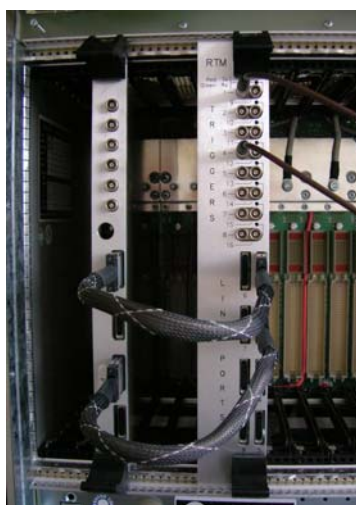
Figure 11: RTM board, one-slot version (left hand side) and two-slot version (right hand side). Two linkport cables connecting the boards are also shown.
